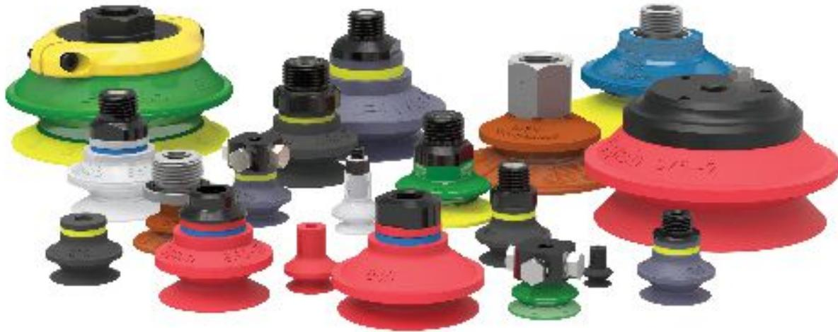
The bellows family is suitable for height differences and slightly uneven or curved surfaces. Several short bellows cups in one lifting device can handle objects with height differences and varying shapes. The bellows also provide a slight lifting movement to separate thin items. This family is available, among other material in FDA compliant material, or the durable DURAFLEX® as Mark Free or even for oily surfaces.
